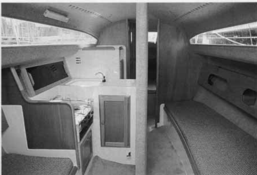
Cabin interior is neatly planned around the lifting centrecase with the galley offset to port.
