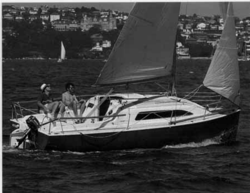
Elliott moving at seven knots on reach shows off its long waterline and powerful hull sections. Design has more fullness forward than is usually the case with this style of yacht.
