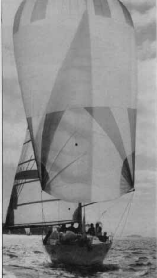
Pig Hunter under light-airs masthead spinnaker. This bow-on view shows the narrow waterline and flared topsides.
