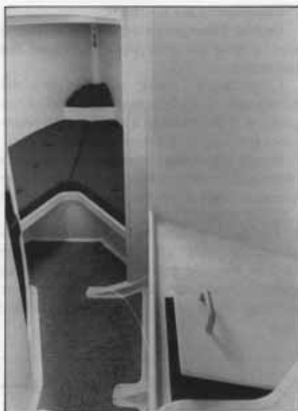
An insert fits into the berth up forward to make a double bunk. To starboard is a fridge and hanging locker. Opposite is the enclosed head.
