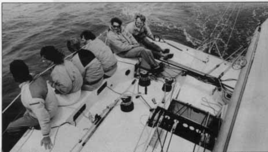
The helmsman has nobody behind him, he is close to both trimmers and space abounds around all controls.
