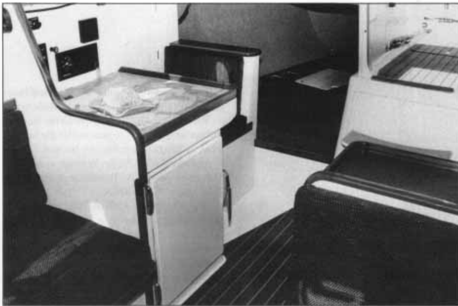
Looking aft on Snap Decision's starboard side shows the double quarter berth and the fridge under the chart table.
