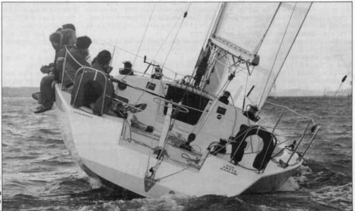
Peacemaker on the warpath upwind . . . flared beam gives helmsman a clear view.
