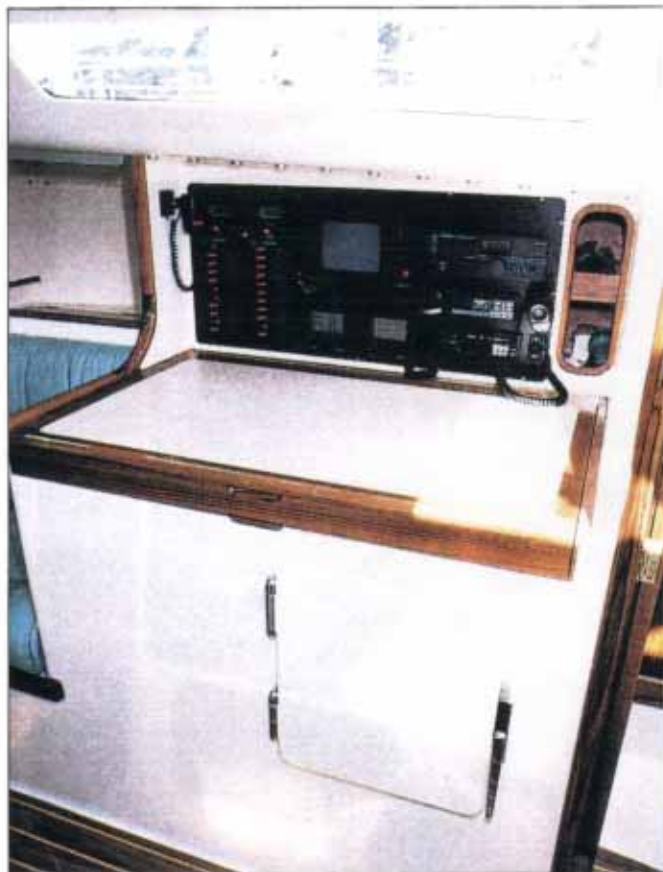
Full instrument package on Total Recall along with dual-lifting tops to the nav table, makes for a tidy navigation/fridge area.
