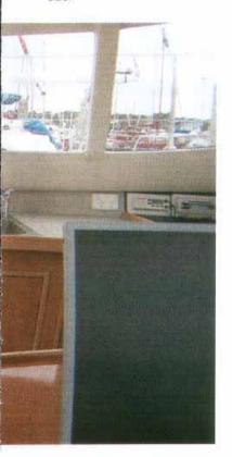
The navigation area still requires some thought because it is quite cluttered and the lifting benchtop obscures the instruments mounted on the outer side. This area was certainly a work in progress at the time of our sail, with a proposal to add a foldout seat and an inverter to be positioned under the navigation station.
