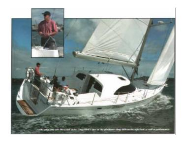
On Elysium the mainsheet is a single loop running through pulleys on top of the pilothouse - and no mainsheet traveller. It relies on a powerful Navtec hydraulic boom vang to keep leech tension on the mainsail and by using this system the usual clutter of traveller, car and mainsheet is removed from the cockpit. The mainsheet can be trimmed by the electric winch.
