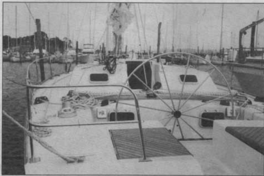
Steering station aft. The large wheel provides finger-tip control and excellent visibility for the helmsman to port and starboard.
