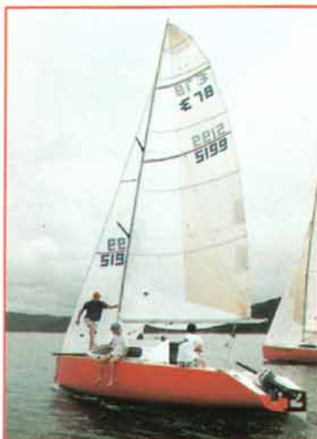
Side decks are curved to provide comfortable seating for the crew.
