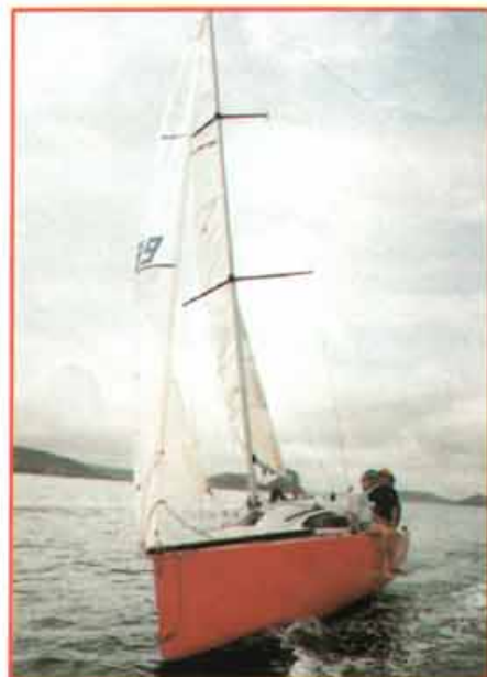
Elliott features simple but highly functional swept-spreader rig with short-footed headsails.
