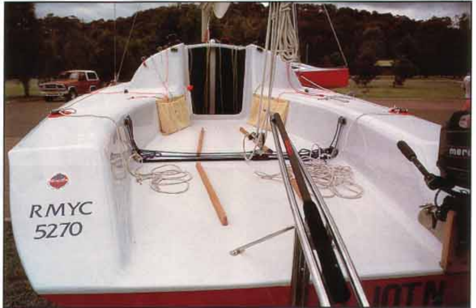
Grand Prix style cockpit keeps crew weight on the gunwale and allows easy boarding from stern.
