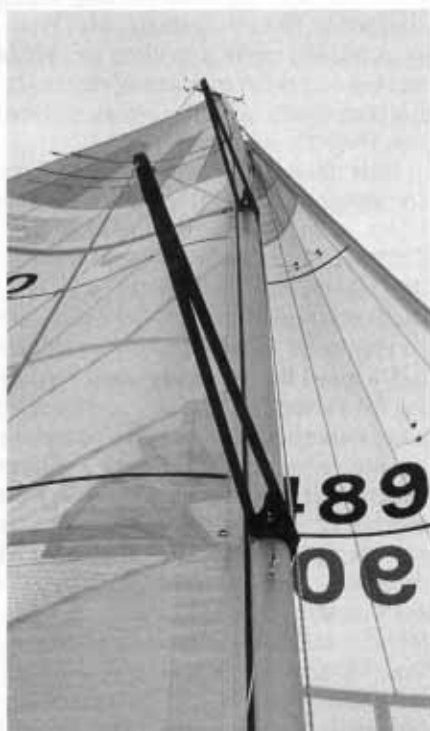
Rig is supported by aft-set caps and lowers over aft-swept spreaders.
