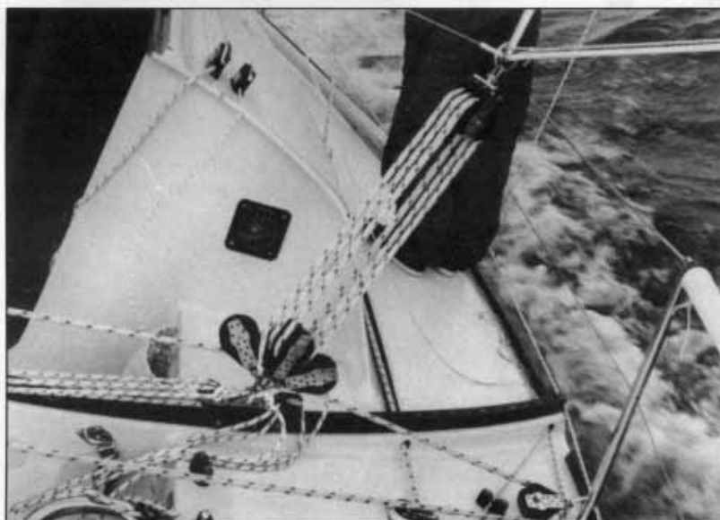
The full-width traveller system allows a large amount of control. The mainsheet is played from the leeward end of the continuous system, which attaches directly to the boom spreader.
