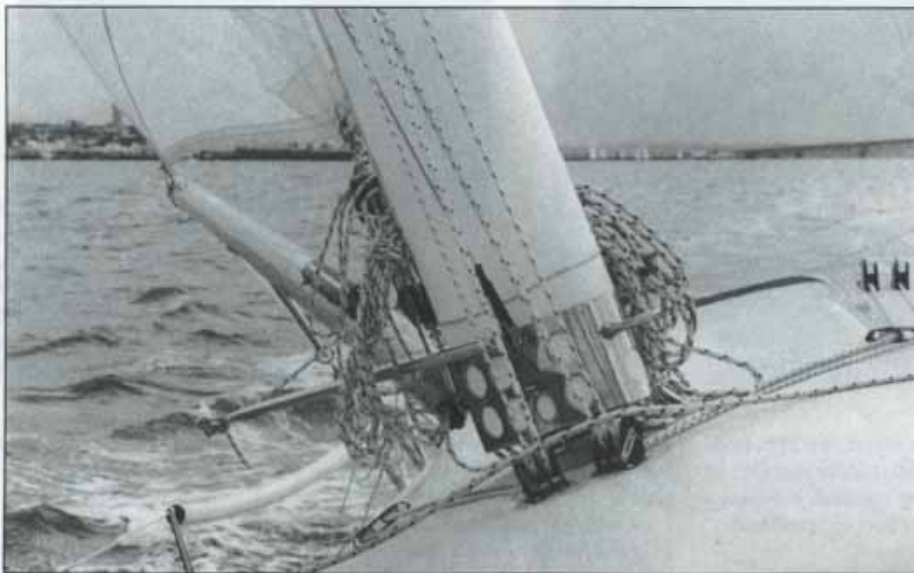
The rotating mast angled for a close reach ... the loose-footed main allows spinnakers to be retrieved over the boom, preventing them from going in the water.
