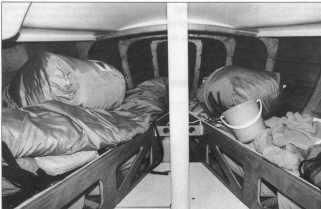
The interior has netting pipe cots supported by the internal box girder bracing system built of foam-ply sandwich.
