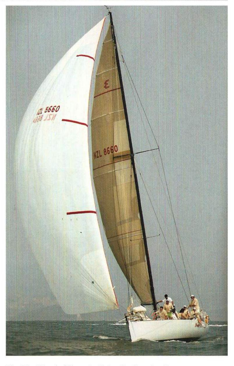
Double-Handed Race in 2002. She has the characteristic Elliott shallow hull shape and low weight that allows her to get out of the water and plane much more quickly than her heavier, deeper competitors. She also has a rotating airfoil-section mast – part of the Elliott philosophy of increasing speed through reducing drag rather than just adding sail area.
