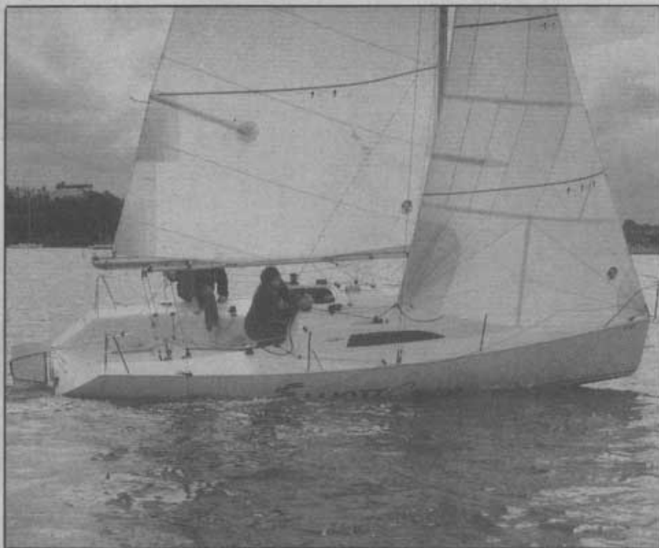
The helm position just forward of the traveller puts everything within easy reach.
